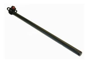
The output of the fluid level sensor is a voltage which changes in direct proportion to the level of fluid in the probe. There are no moving parts. The sensor operates by measuring the capacitance between the probe's two concentric tubes. Due to the difference in permissivity between air and the fluid being measured, the capacitance of the probe changes according to the ratio of air and fluid in the probe.
